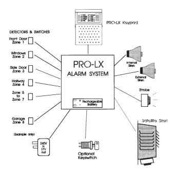
What you will see and use is the PRO-LX Keypad which is set up for you to control the Control Panel and view indicators to find out what is happening. In addition to the keypad may be a key switch or other controls such as push buttons. Your installer will explain the function of all such controls and you will also find them mentioned in the next two chapters.
