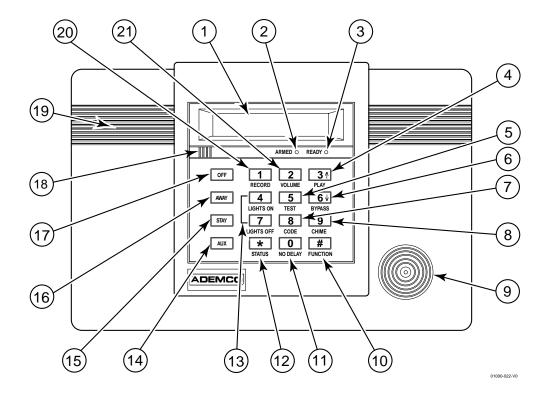
**IMPORTANT!:** When you use the keypad to enter codes and commands, press the keys within 2 seconds of one another. If 2 seconds elapse without a key depression, the entry is aborted and must be repeated from its beginning.
